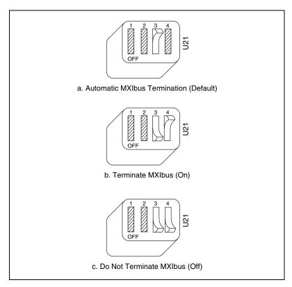
Figure 4-4. MXIbus Termination
